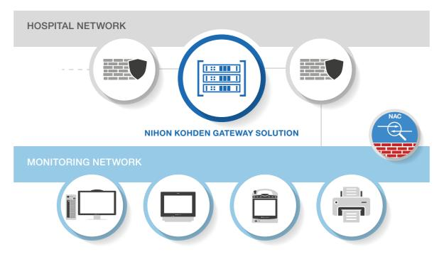
To ensure data integrity and security within the monitoring network, strict traffic segregation is imperative. Nihon Kohden advises physical separation between the monitoring network and client traffic. Employing a divided network infrastructure offers enhanced protection against attacks originating from the client network.
