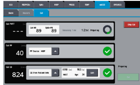
You can visually see which parameter is the reason why the calibration is not proceeding.
